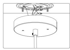
6. Place the Canopy over the outlet box and feed the Fixture Mounting Screws through the canopy openings. Adjust the Fixture Mounting Screws through the nuts until there is enough protrusion out from the Canopy.
