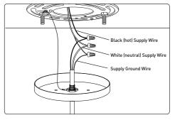
5. Make the following spliced wire connections using wire nuts:
