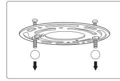
1. Loosen and remove the Ball Nuts from the Round Mounting Plate, set them aside.
