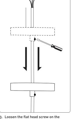
Loosen the flat head screw on the Canopy and adjust the Lamp Cord to your desired length.
