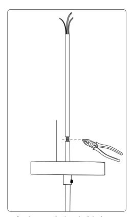
4. Cut the excessive length of the Lamp Cord with a Wire Stripper and reserve a length above the Canopy enough for the hardwire connection.
