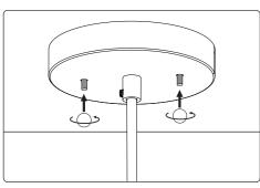
7. Insert the Ball Nuts towards thread of the Fixture Mounting Screws and tighten.
