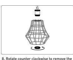
8. Rotate counter clockwise to remove the socket ring from the lamp holder. Attach the cage housing to the lamp holder and rotate clockwise to lock the Socket Ring back to the Lamp Holder.
