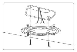
Pull the power supply wires out from the outlet box and install the Round Mounting Plate to the outlet box using the Bracket Mounting Screws included.
