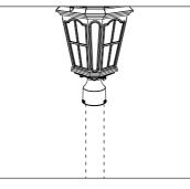
The post lantern can be installed on commercially available 3" round post (not included). Repeat Step 5 thru 9 for installation. Ensure installation is in accordance with NEC and local building code specifications. If not familiar with these codes, consult a certified electrician.
