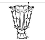
6. Carefully place all the wires and wire connections into the base. Attach the light to the mounting base, and ensure the orientation of the light is correct, with the light sensor facing front. Secure the light to the mounting base with set screws.
