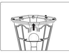
Unscrew to open top cover of post light, and remove the existing light bulb. Only replace light bulb with E26 base, 120 V, 60 W maximum.
