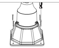
3. Screw the mounting base onto mounting surface. For installation on wood, please use wood screws. For installation on brick or concrete, please use plastic anchor and drywall screws.
