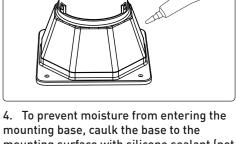
mounting base, caulk the base to the mounting surface with silicone sealant (not included). The sealing compound should fully fill the gap of mounting base and mounting surface.
