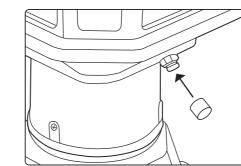
9. (Optional) To turn on the light during the day, place the Cap over the light sensor to disable the dusk-to-dawn feature.
