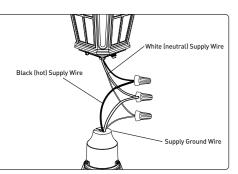
5. Make the following spliced wire connections using wire nuts:
