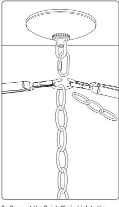
3. Connect the Quick Chain Link to the Chain Holder. Determine the height you want to hang the fixture down from the ceiling. Use a pair of pliers to twist open the chain link end and remove the unwanted portion of chain. Connect the wanted chain to the Quick Chain Link. Twist to close both opened chain links.
