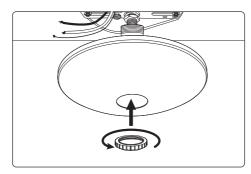
2. Attach the Canopy to the ceiling using the Screw Collar.
