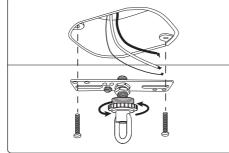
1. Detach the screw collar from chain holder. Mount the Crossbar Kit together with the Chain Holder using the mounting screws.
