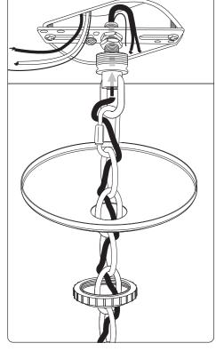
5. Determine the length of wires you need and use a wire stripper tool to cut and strip the wires. Then weave the wires through the chain. Unlock the Collar and release the Canopy to pass the wires through the hole on the Chain Holder and Cross Bar as shown in the diagram.
