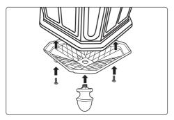
9. Install bottom cap knob onto the bottom cap, and secure the cap to the fixture with bottom cap screws.
