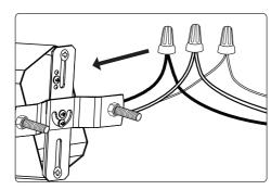
5. Remove the canopy and secure the position of fixture mounting screws by tightening the hex nuts. Carefully place all the wires and wire connections into
