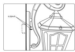
4. Place the canopy over the outlet box and feed the fixture mounting screws through the canopy openings. Adjust the fixture mounting screws until they protrude out from the canopy roughly 1/4 of an inch.
