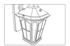
2. Reattach the lower part of the light fixture, and install the rubber washers and mounting nuts.
