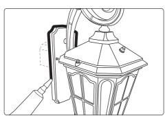
7. After installing the fixture, caulk the upper 3/4 of canopy to the mounting surface with silicone sealant (not included). Leave the bottom 1/4 un-caulked to allow drainage of any water that might leak into the enclosure.
