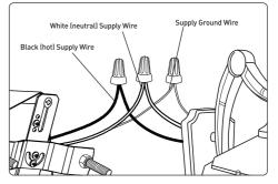
3. Make the following spliced wire connections using wire nuts:
