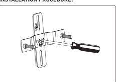
1. Unscrew the lock nuts from the mounting bracket.
