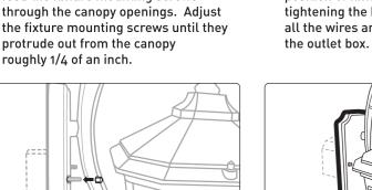
6. Place the canopy over the outlet box with fixture mounting screws feeding through the openings. Install the rubber washers first, then install the canopy mounting nuts.
