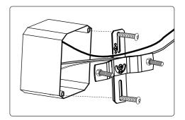
Pull the power supply wires out from the outlet box, and install the mounting bracket to the outlet box using the bracket mounting screws.
