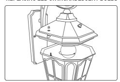
1. Open the coach light fixture body by unscrewing the mounting nuts and rubber
