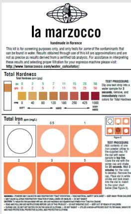
The parameters that you can measure are Total Hardness, Total Iron, Free Chlorine, Total Chlorine, pH & Total Alkalinity, Chlorides.
