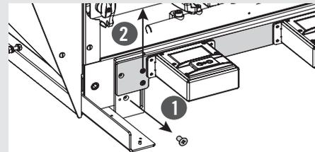
To remove the electronic box you need to remove the drain tray, unscrew and remove the lower screws ①, loosen the upper screws ② without removing them and move the scale crosspiece up. Now you can access the electronic box or remove it.
