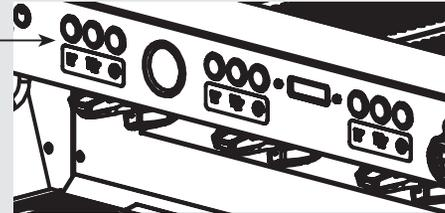
The keypad has two functions. The first is for control of the espresso. The second is for programming individual software parameters. The programming of the individual parameters is possible only using the buttons in the group 1 (group starting from the left).
