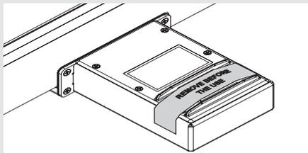
Don't spill water onto the scale box. If needed, gently remove it with an absorbent cloth. Should any water and/or dirt penetrate into the holes highlighted
