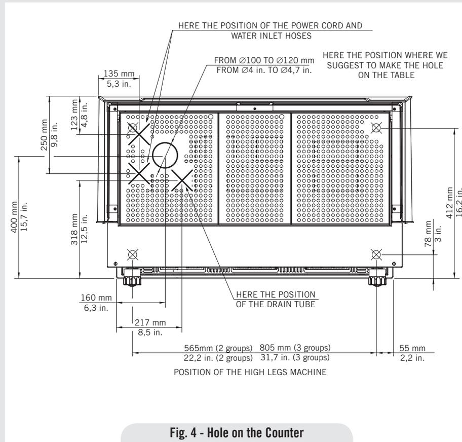
Fig. 4 - Hole on the Counter
