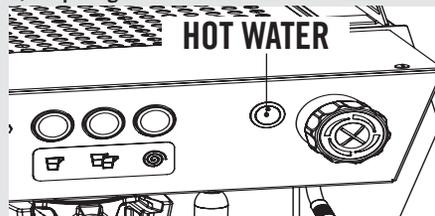
You may dispense hot water by using the fixed nozzle (item 9 fig 1). To dispense hot water, press the hot water button on the right most group.
