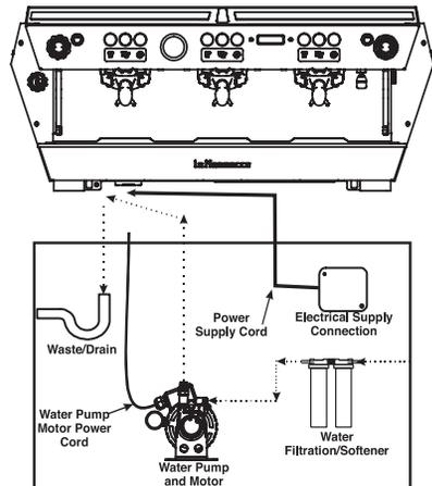
Fig. 2 - Installation Guide
