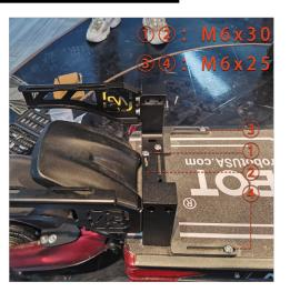
3Aligning the bracket with the center mount, and then tighten the fixing bolt with a 6mm hex wrench according to priority. (Screw x4)
