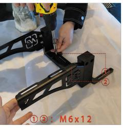
②Tighten the screws with a 6mm hex wrench. (Screw x2)
