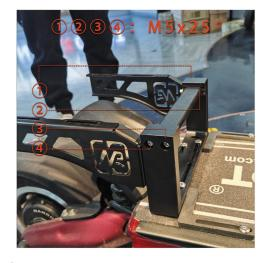
(4) Tighten the screws with a 5mm hex wrench. (Screw x4)
