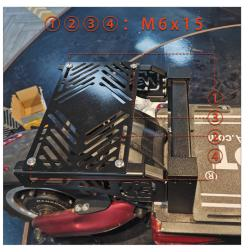
⑤Tighten the screws with a 6mm hex wrench according to priority. (Screw x4、Nutsert x4)
