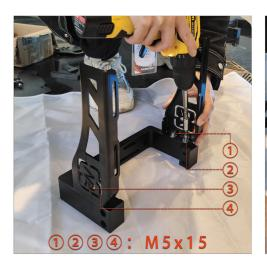
①Tighten the screws with a 5mm hex wrench,which is included in the basic tool kit.
