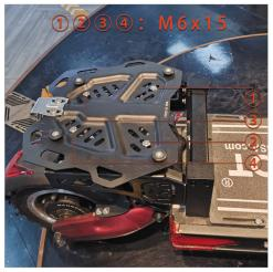
6 Tighten the screws with a 6mm hex wrench according to priority. (Screw x4、Nutsert x4)
