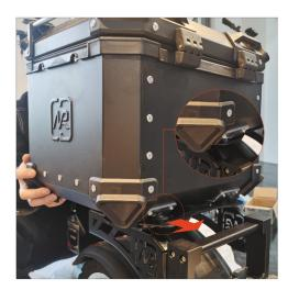
Taligning the trunk with the center mount, and then push the trunk for -ward until it snaps.
