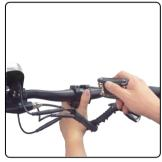
2. AFTER ALIGNING THE HANDLEBAR WITH THE CENTER MOUNT, REPLACE THE COVER MOUNT, AND TIGHTEN THE FIXING BOLT.
