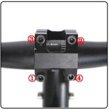
3. PROGRESSIVELY TIGHTEN THE BOLTS IN SEQUENTIAL ORDER (1 TO 4), ENSURING THERE IS EQUAL DISTANCE BETWEEN THE MOUNT AND HANDLEBAR ENDS.
