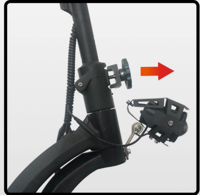
② Keep loosening the folding knob until the J-shaped buckle completely leaves the grooves
