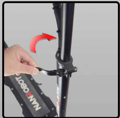
④ The silver fixing buckle clasps the height hole, tighten the fastening buckle and turn it back in the direction of the arrow
