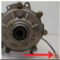
\*\*Only use this connector with the wire jumper if your differential has this 2 pin connector\*\*
