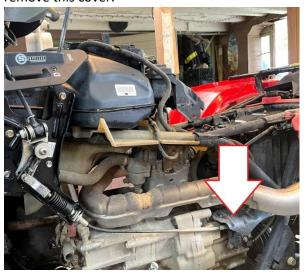
19) Adjust these two nuts on this cable so the Low gear shifter will shift between L and D:
