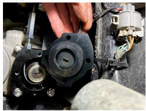
28) Push the switches housing onto the actuator so the flat blade in the switches housing slides into the slot in the actuator.
