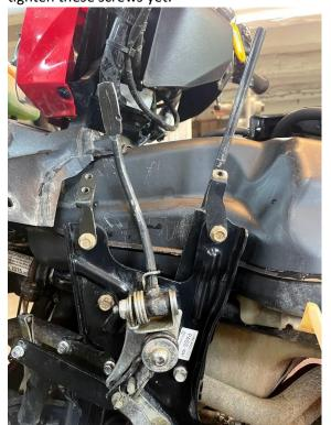
16) Install the plastic shift guide using the 3 button head screws, tighten these down evenly so the brackets are flat against the shift guide. Then tighten the bracket screws:
