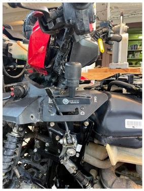
23) Unscrew the adjuster on the actuator until the notch marks line up. Only make adjustments when the lever is in the 4wd position. This is the 4wd position:
