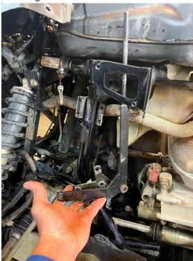
12) Use the plastic push fastener to align the lever bracket with the frame and hold it in place.
