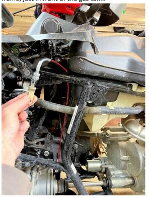
7) Install the thin frame bracket using one 1/4-20 screw to hold the back side together, then unscrew one of the nuts on the cable and push the cable through the slot in the metal brackets. Use the two nuts on the cable to tighten the bracket to the frame, do not over tighten these. Screw in the 1" long 10/32 screw so it is pinned against the frame, this will hold the bracket from rotating, do not over tighten:
