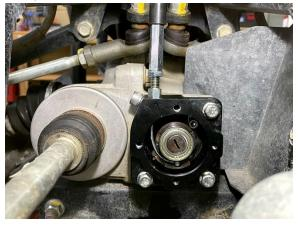
24) Shift into diff lock, if it will not move all the way you must raise the front wheels off the ground and rotate the wheel while pushing on the lever. This action gets the gears inside the differential to move and line up so they can slide together. Do not force the lever. This is the shifter position and actuator position when in diff lock:
