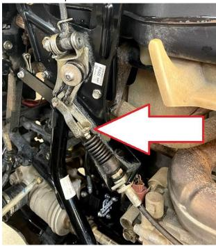
18) At the other end of this cable is a metal cover, remove the two screws holding it on and remove this cover:
