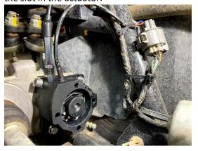
29) Put the O-ring on the lid and screw the lid and switches housing onto the actuator using the long 1/4-20 screws provided.
