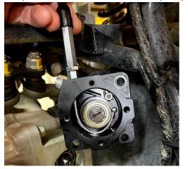
4) Rotate the shaft in the differential clockwise as far as it will go, do not force it, then rotate it CCW a little so it is vertical which will match the manual actuator:
