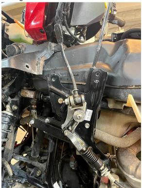
15) Attach the Shift Guide brackets to the Low Gear shifter using the new supplied screws, do not tighten these screws yet:
