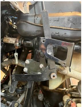
13) Attach the cable to the shift lever. Using the 10-32 x 1" long screw put a washer on it, then slide it through holes on the bracket on the end of the cable. Next put a washer on and then a nut, put this nut on so the flange is facing the end of the screw, slide the bolt through the shift lever bracket and then put the other nut on the screw. Tighten the nuts so the screw is flush with the end last nut. This is what the assembly will look like:
