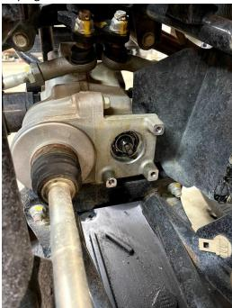
3) Screw the pull cable into the manual actuator and put the ball of the cable into the pulley:
