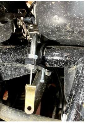
8) Install the large frame clamp, if the U bracket is loose on the frame stick the strip of rubber to it. Then use the push fastener to line up and hold the bracket in place. Install 3 of the 4 screws, do not tighten these yet:
