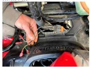
26) Plug in the 8-pin connector to your wire harness (If you purchased the Display Lights Upgrade Kit this connector will have a yellow wire connecting two terminals. Otherwise, all the holes are plugged)
