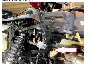
12) Attach the cable to the shift lever. Using the 10-32 x 1" long screw put a washer on it, then slide it through holes on the bracket on the end of the cable. Next put a washer on and then a nut, put this nut on so the flange is facing the end of the screw, slide the bolt through the shift lever bracket and then put the other nut on the screw. Tighten the nuts so the screw is flush with the end last nut. This is what the assembly will look like:
