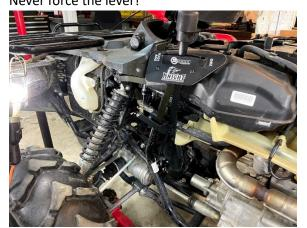
15) Unscrew the adjuster on the actuator until the notch marks line up. Only make adjustments when the lever is in the 4wd position. This is the 4wd position:
