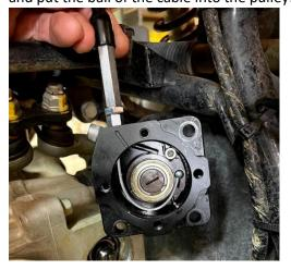
4) Rotate the shaft in the differential clockwise as far as it will go, do not force it, then rotate it CCW a little so it is vertical which will match the manual actuator:
