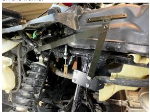
11) Screw the shift lever into the flat bracket, do not remove any of the nuts or washers from the bolt on the lever, they are meant to be there, simply screw it in:
