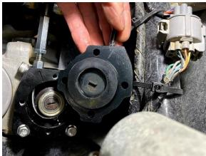
20) Push the switches housing onto the actuator so the flat blade in the switches housing slides into the slot in the actuator.
