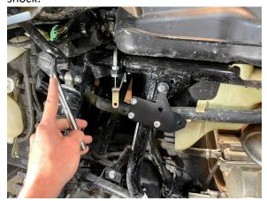
10) Reuse this bolt and install the long bracket, attach it to the T bracket using the button head screw, attach the T bracket to the flat bracket on the frame:
