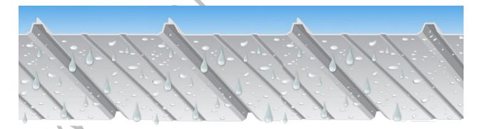
Sometimes under the right circumstances, condensation can occur with only a few degrees difference between the inside and the outside temperature. Under these conditions it's almost impossible to totally eliminate condensation without adding some additional heat to the inside surface. Remember the example above where we talked about how using the hair dryer warmed up the cold surface of the mirror?
