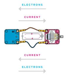
Circuit Cubes are stackable, so the poles can be touching from below as well as next to each other, depending on how one connects them. When the Battery Cube is switched off, it makes a gap in the circuit and the electrons are not able to flow around. When the switch is turned on, it closes the gap and the electricity can move and make the Cubes work again.
