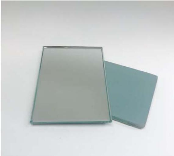
Copper-free mirror is made by thoroughly cleaning annealed glass and sensitizing it with a diluted solution of tin chloride. Silver nitrate is sprayed onto the surface of the glass along with other proprietary chemical configurations. After silvering, a two-coat paint system is applied to encapsulate the formula with low-lead or lead-free solution along with a copper-free paint solution.
