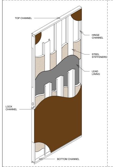
Lead Glass Pro Hollow Metal Lined Doors are manufactured with 16 gauge A60 galvanneal steel and internally steel stiffened.
