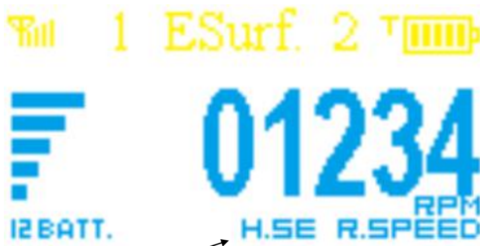
Motor RPM is detected by one hall sensor wire.
