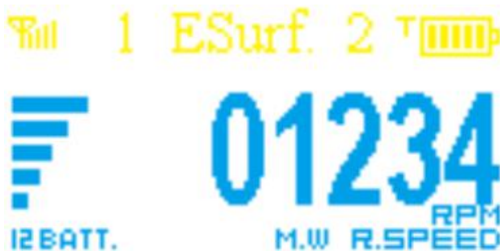
Motor RPM is detected by one Motor phase wire.
