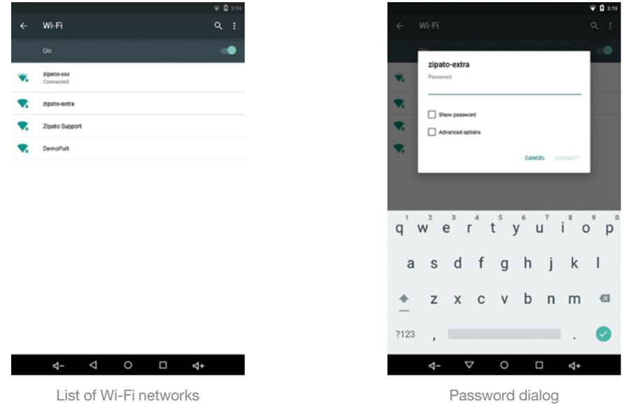
Some wireless networks do not broadcast their names (SSID). In that case, select three dots in the upper right corner and choose Add network from dropdown menu. To make the connection, type the network name (SSID) and follow the above procedure from step 4. When setup completes, Wi-Fi Connected icon appears.
