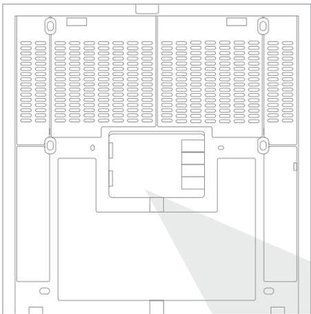
In addition to range of wireless technologies ZipaTile also offers connection to wired equipment at the back of the device. This includes external temperature sensor (not included), one input and two outputs or three outputs (depending on version) for controlling relays (please note max. voltage and current) or for signaling to boilers, heating or irrigation equipment.
