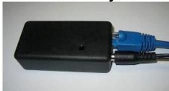
The Mi-Gateway-1 receives wireless messages from multiple Mi-Sensor-1 sensors and sends them to an email account or text message to a phone using your Local Area Network (LAN) to Internet connection. The Mi-Gateway-1 has a built-in web server that is accessed with any web browser to configure all parameters of the Mi-Gateway-1 and Mi-Sensor-1. The Mi-Gateway-1 plugs into your LAN and is powered from an AC outlet.
