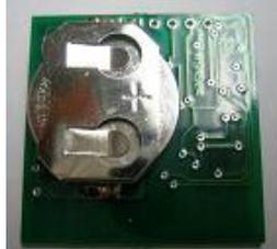
Open sensor by prying case open by hand. Insert CR2032 battery in holder ensuring to observe polarity indicator on battery and battery holder.
