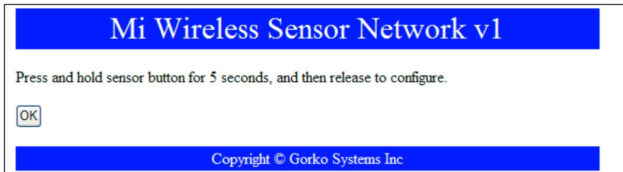
Selecting the OK button will cancel the Configuring mode and take the user to the STATUS screen where if a sensor is correctly configured a Config Report Type will be displayed for the configured sensor. If you do not see a Config Report Type, the sensor test button was not held for greater than 5 seconds, or the sensor is out of range.
