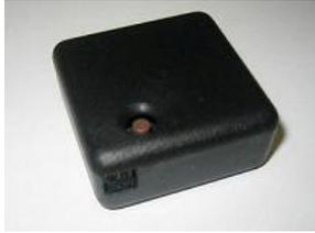
The Mi-Sensor-1 is a multifunction battery powered wireless sensor capable of simultaneously monitoring Temperature, Motion/Shock, Button Press, Presence and one port function consisting of Contacts or Moisture/Water or Humidity or Light or Milli-volts AC or Milli-volts DC or Capacitance or Amp Hours.
