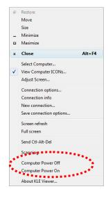
Now you can use the Viewe Quick Menu to perform power on / power off command remotely across internet by using the TK-IP101 together with an TK-RP08.
