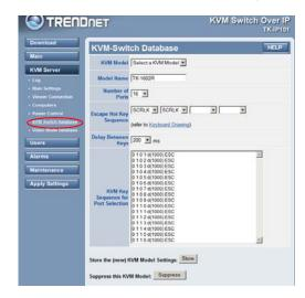
The various settings on this page are KVM port-specific because a computer is first identified by the KVM port it is attached to. Select the target port on which your subsequent settings on this page are directed. You can use the drop-down combo box as well as use the *Previous* and the *Next* button to navigate to a specific port.
