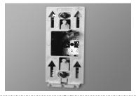
6. Pass the wires from the wall through the hole at the base of the mounting base and connect them using the solderless connectors supplied. When making the connection with aluminum wire, make sure that you are using connectors identified CO/ALR. Please note that the thermostat wires do not have polarity. Therefore, the way they are connected is not important.
