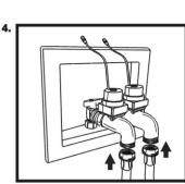
5. Lightly wrench tighten all connections 1/4 turn, or until snug. Do not over tighten.
