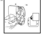
8. With the contacts of the wire harness connector facing you, plug the 6-pin connector end of the Wire Harness into the bottom of the Control Panel.
