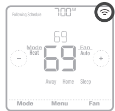
Example of thermostat included and connected in a Z-Wave network.
