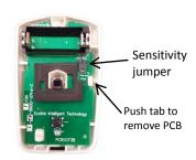
tight seal around the knockouts to prevent bugs from entering the sensor and causing false alarms. Replace the circuit board and snap the front cover onto the back cover.
