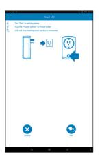
Plug the Power Switch into a standard AC outlet having 120V, 60Hz; the LED will blink indicating the Power Switch is in the pairing mode.
