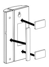
Select a location on a door or window. The large section of the sensor should be fixed on the immovable frame of the door/window.
