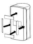
Select a desired location. It is recommended to place the Motion Detector in the corner of the room and between 6 to 8 feet from the floor. See notes in step 2 of the top of the next page for installation recommendations.
