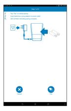
The App will then search for the Indoor Siren. If the App did not detect the Siren, press the Pair button located inside the battery compartment in the back.
