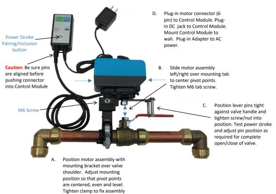
3. Mount motor assembly on to valve:
