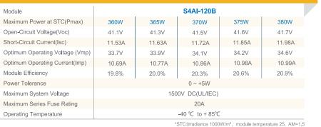
\*STC:Irradiance 1000W/m², module temperature 25, AM=1.5 Optional black frame or white frame module according to customer requirements
