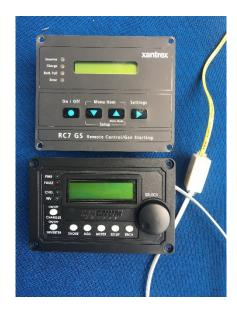
Remove the OLD cable from the back of the RC7 remote. (phone cord, usually yellow) Plug the adaptor into the old cable on one end. Plug the other end into the NEW RC50 remote.
