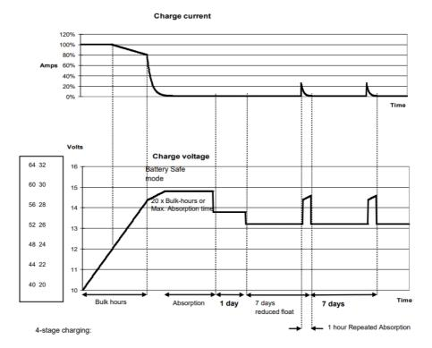
Bulk-mode: Entered when charger is started. Constant current is applied until the gassing voltage is reached (14.4V resp. 28.8V, temperature compensated).
