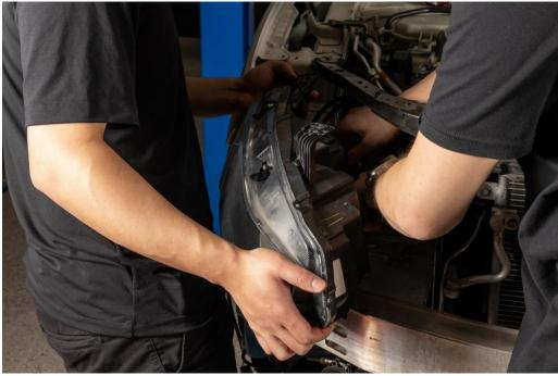
13 – Set your OEM headlight assemblies on a work surface. You will need to transfer the bumper brackets attached to them over to your new OLM headlights. There are 2 10mm bolts on the bottom of the housing. Tighten the bolts to 6.9Ft-Lbs or 9.4Nm.
