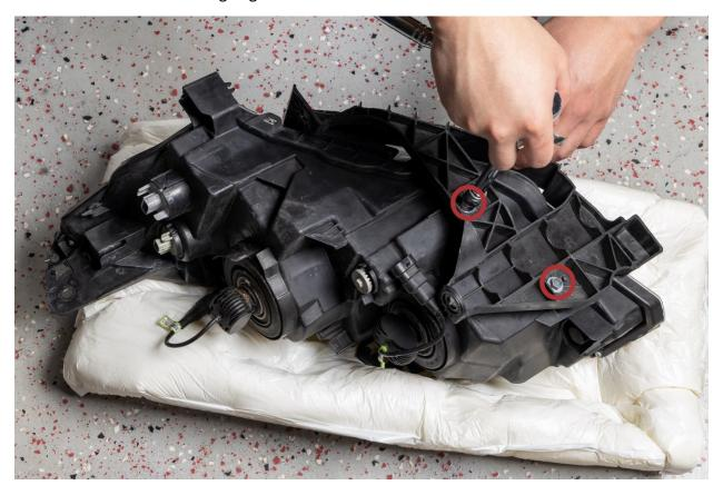
14 – On the front of the OEM housings are 2 clips that help secure the bumper. Remove the phillips head screws and reinstall install to your OLM assemblies. Set aside for installation.
