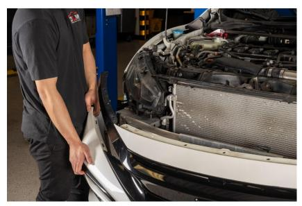
10 – There are 2 10mm bolts along the crash beam that need to be removed:
