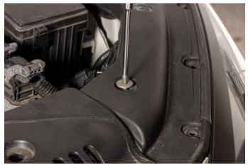
3 – Remove the hood seal trim that overlays the headlights and front edge of the bumper cover.
