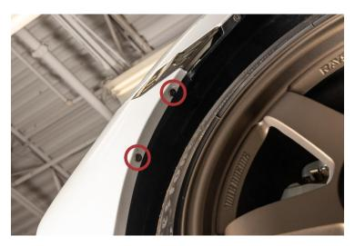
6 – You will need to remove the side markers from the vehicle. By removing the previous 2 screws, the wheel liner should be able to be peeled back for access to the back side of the sidemaker housing.
