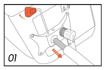
Push the lever up and check if the gas lift is fully extended.
