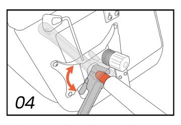
Twist back and forth until the gas lift is released.
