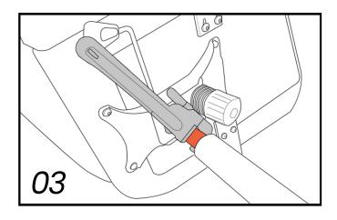
Tightly fix the wrench on the thin part of the gas lift.
