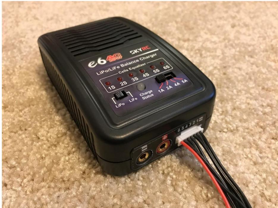
Once you have followed through these steps, you will notice the six 1S-6S lights glow red and occasionally blink. The Charge Status light will glow red when charging, orange when almost charged, and green when the Ibex2 is done charging. Only unplug the Ibex2 from the charger when the Charge Status light glows GREEN.
