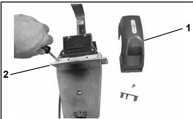
Single Lever Remote Control 1. Remote control cover 2. Flange
