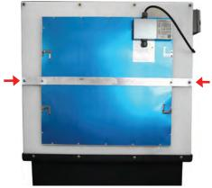
Attach light fixture to the top of the washout booth using 2-1/2"SS Pan Head Bolts (G)
