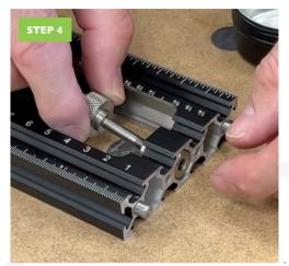
Take a thumbscrew and place it in and through the bush, fixing it into the T-Nut and lock this into place. Apply this on all 4 of the extrusions.
