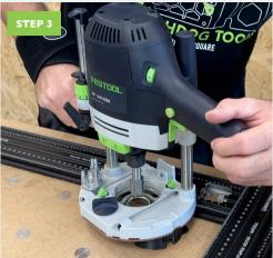
When you are routing, the puck will slide around on the router and make sure that this does not tip.
