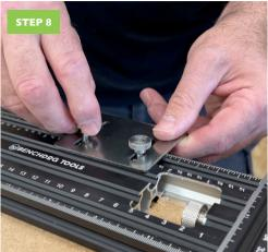
Once you have the angle stop attached to the jig you can slide the angle stop up and down to where you want the stops to be, and then tighten them down giving you a nice and straight reference edge.
