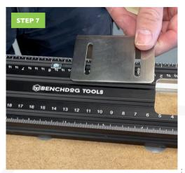
Using the angle stop, bring the router to the edge of the table and then apply the thumbscrews.
