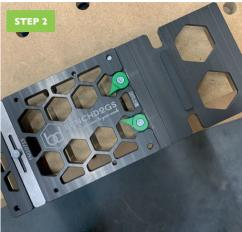
Place the square/rail over the bevelled edge of your work piece to enable you get maximum stability to make the cuts you require.
