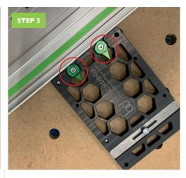
Slide your rail through the guide on the square and tighten the thumbscrews to secure the rail in place - this setup will enable you to cut at 45° angles.
