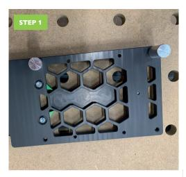
Screw either the 30mm Bevel Adapters or the 60mm adapters – depending on the thickness of the board you are cutting – into the holes as shown.
