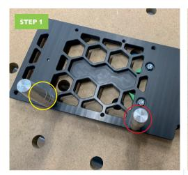
You will need 1x MFT grooved 45° adapter which can be bought separately. Screw one MFT grooved dog in the right hand hole (marked red) and a MFT grooved 45° adapter in the smaller hole on the left (marked yellow).
