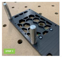
Screw the MFT grooved dogs in the holes as shown.
