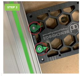
Slide your rail through the guide on the square and tighten the thumbscrews to secure the rail in place - this setup will enable you to cut at 90° angles.
