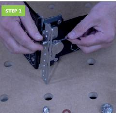
Using the supplied allen key, tighten the fixing screw to the alignament pin.
