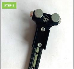
Attach the track adapter bar to the track adapter using the thumbscrews provided. Leave slightly loose to enable fitment to your rail.
