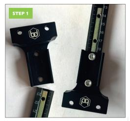
Take advantage of this feature, flip your track adapter over and attach to the underside of your guide rail (the side displaying the narrow cut markings) using the provided hex bolts. Leave loosened to adjust
