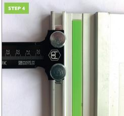
With your thumbscrews loosened, slide your track adapter into the fitment on your rail, when placed at the desired position, tighten the thumbscrews to secure.
