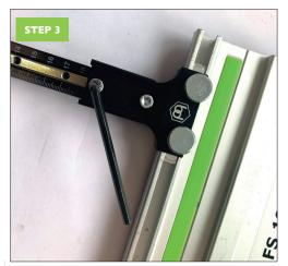
with your thumbscrews loosened, slide your track adapter ito the fitment on your rail, when placed at the desired position, tighten the thumbscrews to secure. Adjust the rail to your desired cut (displayed at the edge of the track adapter) and secure using the hex bolts.
