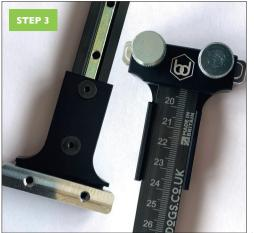
Attach the track adapter bar to the track adapter using the thumbscrews provided. Leave slightly loose to enable fitment to your rail.
