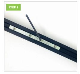
Join the rails using the joining bars. Tighten using the supplied Allen Key.
