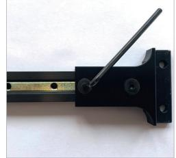
Attaching the Track Adaptor to the rail using the a joining bar. Place the bar in the rail as per below. Using the Countersunk screws tighten the adapter onto the rail.
