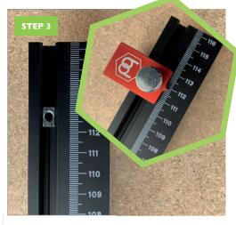
Slide the t-nut into the guide, attach the aluminium stop and move to the desired position. Once positioned tighten the thumbscrew.
