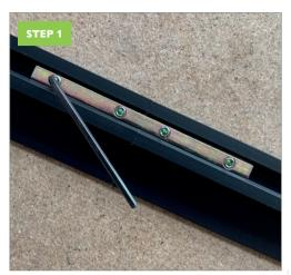
Join the rails using the joining bars. Tighten using the supplied Allen Key.
