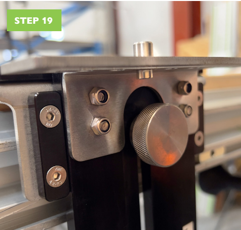
Insert this in the hole in line with the brand you have ordered (FMTE - Festool Makita Triton and Evolution)
