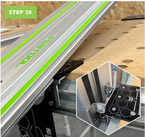
Check hinge lifts into a vertical position and stays in place with the hinge in its upright or lowering position, there will be some lateral movement this is normal and will not move once located in the alignment pin
