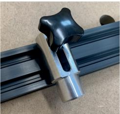
Slide the t-nut into the fence as shown below and screw the Fence Dog into the t-nut using the thumbscrew.
