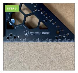
Turn over your carpenter square and place so the alignment pins are touching the edge of your sheet. This will allow you to make accurate markings at 6mm, 7.5, 9 and 12.5mm from the edge.
