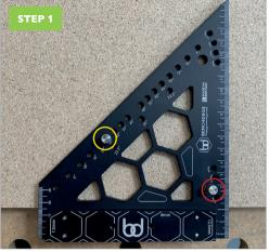
Using the supplied alignment pins, screw the first pin (RED) in the hole marked 'PIVOT' and the second pin (YELLOW) in the hole marked with your desired angle.
