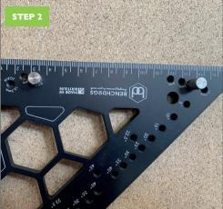
Choose your desired measurement and screw in the supplied alignment pins in the matching marked holes.
