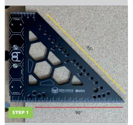
Place the carpenter square so the cheek is touching the side of your sheet. Using either the straight or diaganol edge, make your markings at either 90° or at 45°.
