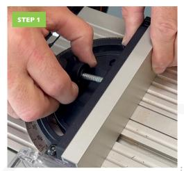
Remove the thumbscrew and fence that comes with the CSC SYS 50 table saw. Put the fence somewhere safe and keep the thumbscrew as you will need this later.
