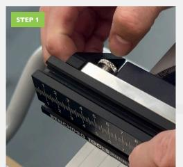
Slide on the guard lifter to the end of the fence that is near to the cutting blade and this will allow you to glide this through the safely guard without any snagging.
