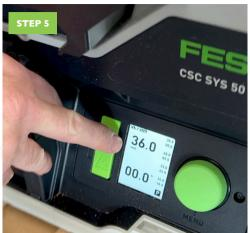
Next you need to set the hight of the blade to be at a minimum of 36mm. This allows the fence to go through and return back.
