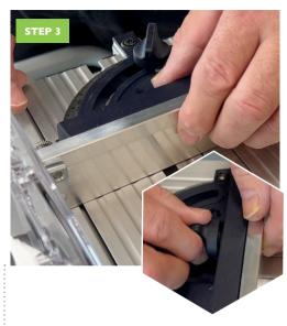
Taking the adaptor plate, align up this against the mitre saw. Using the thumbscrew that is supplied with the CSC SYS, screw this the adaptor plate into position and making sure that this is nice and tight.
