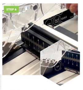
You then want to make sure that you are 1mm away from the saw blade. This can be done using a1mm set up block and putting the set up block up against the blade and the fence and then sliding the fence up against it, giving you the perfect distance away from the blade. Tighten up the thumbscrews on the adaptor plate and that is now set.
