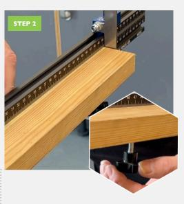
Place the material on top of the support plate and you can adjust the thumbscrew underneath if you need to align and level the material out.
