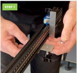
For the 625mm and 1000mm Fence, you can slide the material support plate on the underside of the extrusion and screw them into place using the attached thumbscrews. This is for when the material you are using is large / long to stop the material from tipping.
