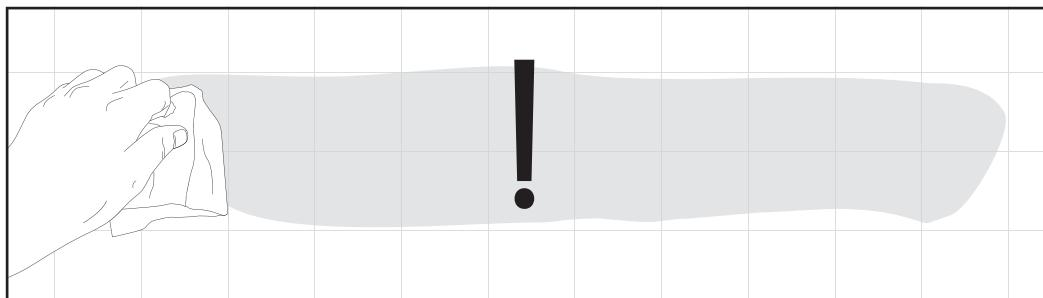
**2** Apply Silicone to back of Shelf & peel off paper backer from pre-applied Tape.
