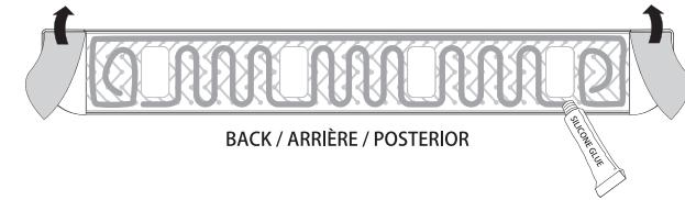
**3** Press Shelf firmly against the wall for 10 seconds. Wait 24 hours for Silicone Glue to cure before proceeding to use the shelf.
