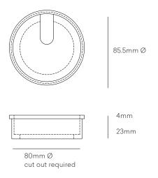
American oak DIMENSIONS 85.5mm Ø TIMBER FINISHES Clear lacquered Raw (unfinished) STONE FINISHES Bianco 10mm Verde 10mm Peach & grigio 20mm Travertine 20mm Viola 20mm NOTES Ø Diameter of the product Install 80mm cut out required Flange cover overhangs 2.5mm to cut out
