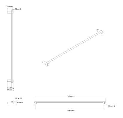
MATERIAL Stainless steel (SS304) DIMENSIONS 945mm L 80mm P FINISHES Brushed gold Brushed satin Matte black Polished chrome NOTES Overall length of the towel rail Projection Fixing Fixings and install instructions included in package SS304 304 grade stainless steel
