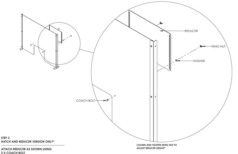
ATTACH REDUCER AS SHOWN USING: 2 X COACH BOLT 2 X WASHER 2 X WING NUT
