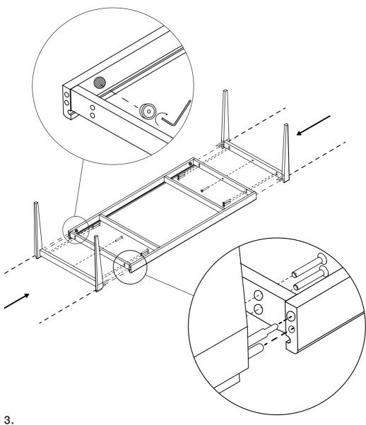
Connect the legs to the frame using supplied screws.
