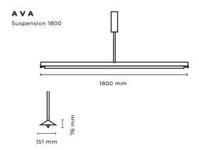
Туре Pendant light Material Solid brass Environment Indoors Dimensions 1800 x 151 x 76 mm 70.86 x 5.94 x 3" Weight 18 kg; 39.7 lb Ceiling rose Ø 90 mm x 205 mm
