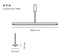
Pendant light Туре Material Solid brass Environment Indoors Dimensions 1500 x 151 x 76 mm 59.05 x 5.94 x 3" Weight 14,5 kg; 32 lb Ceiling rose Ø 90 mm x 205 mm Ø 3.54" x 8.07"
