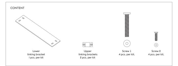
Use screw 1 x 2 to attach the lower linking bracket as illustrated to one fully assembled section.
