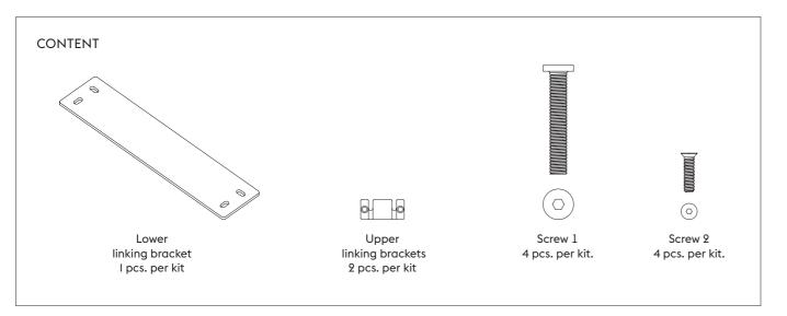
Use screw 1 x 2 to attach the lower linking bracket as illustrated to one fully assembled section.
